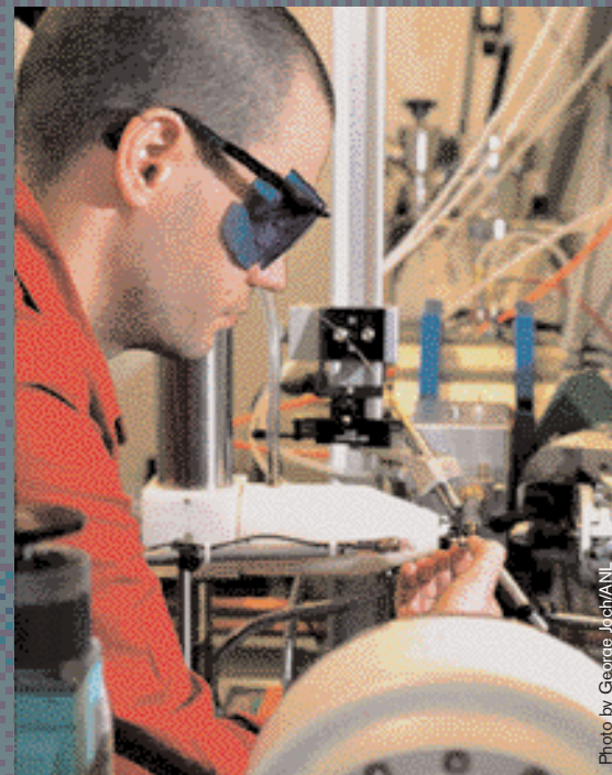
Donning laser safety glasses, scientist Spencer Anderson secures a glass capillary tube that contains a PYP protein crystal to the "molecular camera" in an APS research lab at Argonne.
